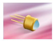
Opto Diode offers the high output red LED in a hermetically-sealed TO-5 can with three leads. Under absolute maximum ratings at 25 degrees C, the continuous forward current is 500 mA, with reverse voltage of 10V. The lead soldering temperature (1/16 inch from the case for 10 seconds) is 260 degrees C, making this LED easy and convenient to install into new and/or existing lighting systems.
